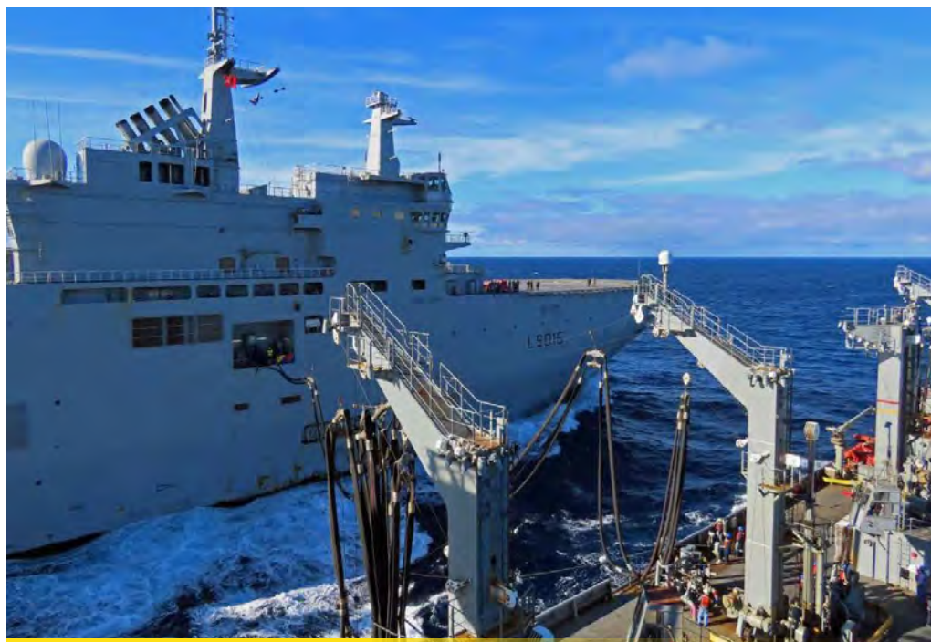
U.S. Navy's Military Sealift Command USNS Laramie (T-AO 203) completes a refueling-at-sea with French Navy amphibious assault ship Dixmude (L9015) in the Atlantic Ocean. (U.S. Navy photo by Thomas Epps)
