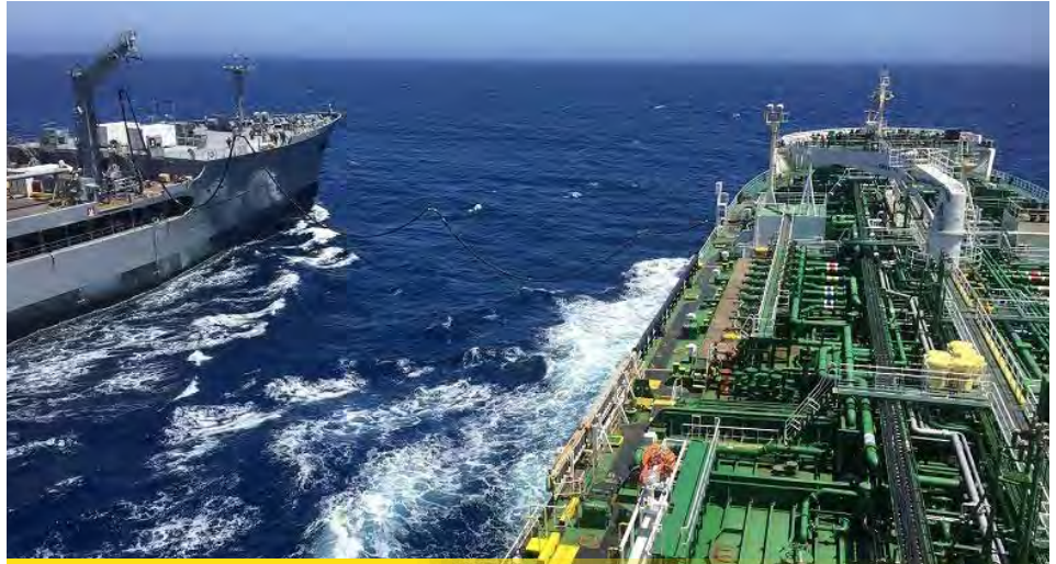
Military Sealift Command fleet replenishment oiler USNS Yukon (T-AO 202) conducts a consolidated cargo replenishment (CONSOL) at sea with the MSC long-term chartered motor tanker ship MT Empire State (T-AOT 5193). (U.S. Navy photo by Sarah Burford).
