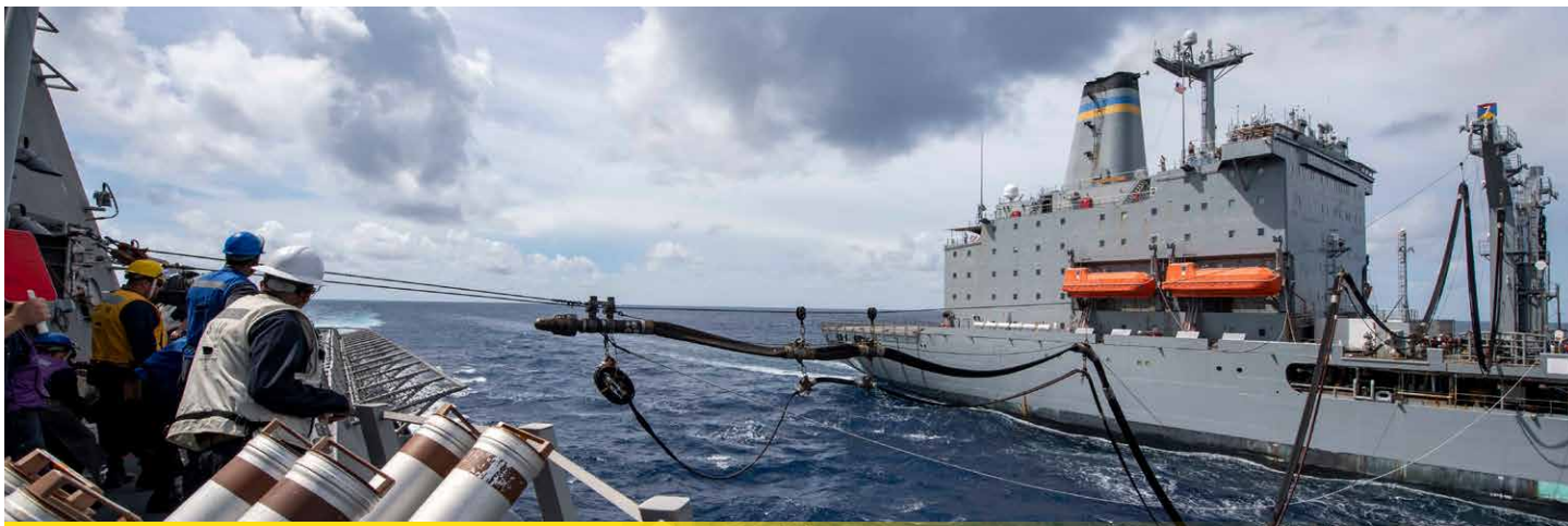
Sailors prepare for the probe to seat during a refueling-at-sea aboard Independence-variant littoral combat ship USS Charleston (LCS 18), and Henry J. Kaiser-class underway replenishment oiler USNS Tippecanoe (T-AO 199). (U.S. Navy photo by Mass Communication Specialist 3rd Class Adam Butler)
