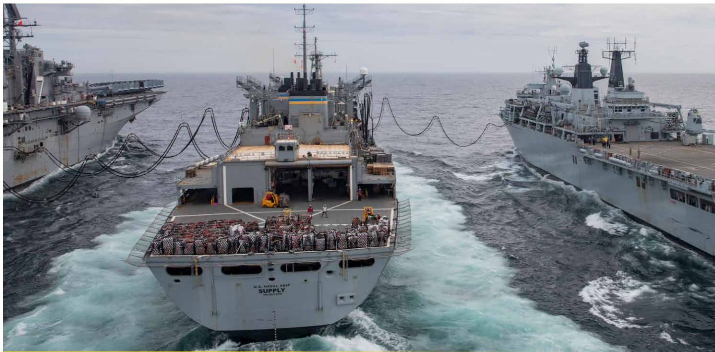
The Wasp-class amphibious assault ship USS Iwo Jima (LHD 7), left, the fast combat support ship USNS Supply (T-AOE 6) and the Royal Navy landing platform dock ship HMS Albion (L 14) conduct a replenishment-at-sea. (U.S. Navy photo by Mass Communication Specialist 3rd Class Jessica Kibena)
