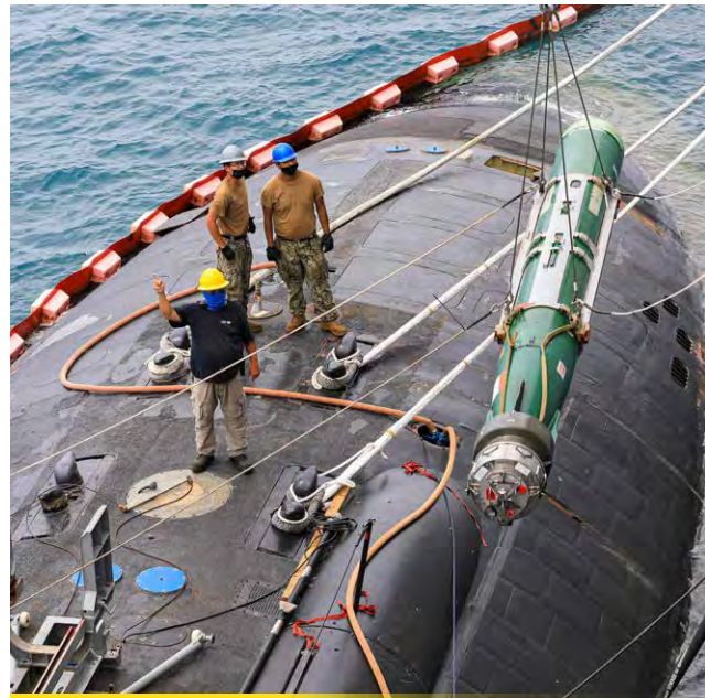
Sailors and civil service mariners assigned to the submarine tender USS Emory S. Land (AS 39) and Sailors assigned to the Los Angeles-class fast-attack submarine USS Asheville (SSN 758) offload a Mark 48 advanced capability torpedo from Asheville during a weapons handling evolution. (U.S. Navy photo by Mass Communication Specialist 3rd Class Naomi Johnson)
