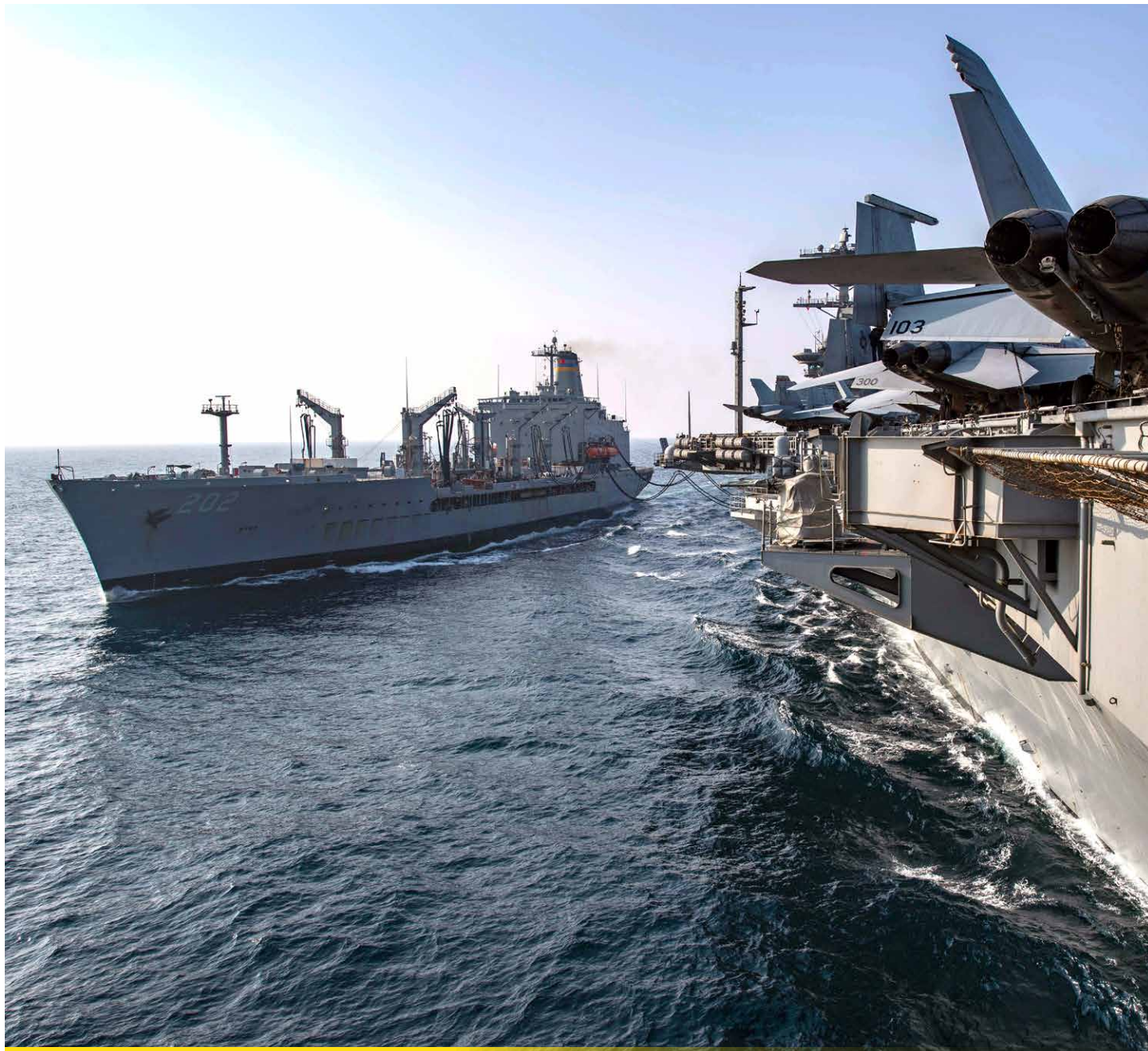
The Henry J. Kaiser-class underway replenishment oiler, USNS Yukon (T-AO 202), steams alongside aircraft carrier USS Nimitz (CVN 68) during a replenishment-at-sea. (U.S. Navy photo by Mass Communication Specialist 3rd Class Charles DeParlier)
